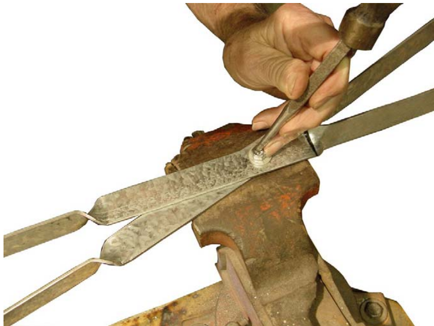
Figure 15 Locking the nut.
