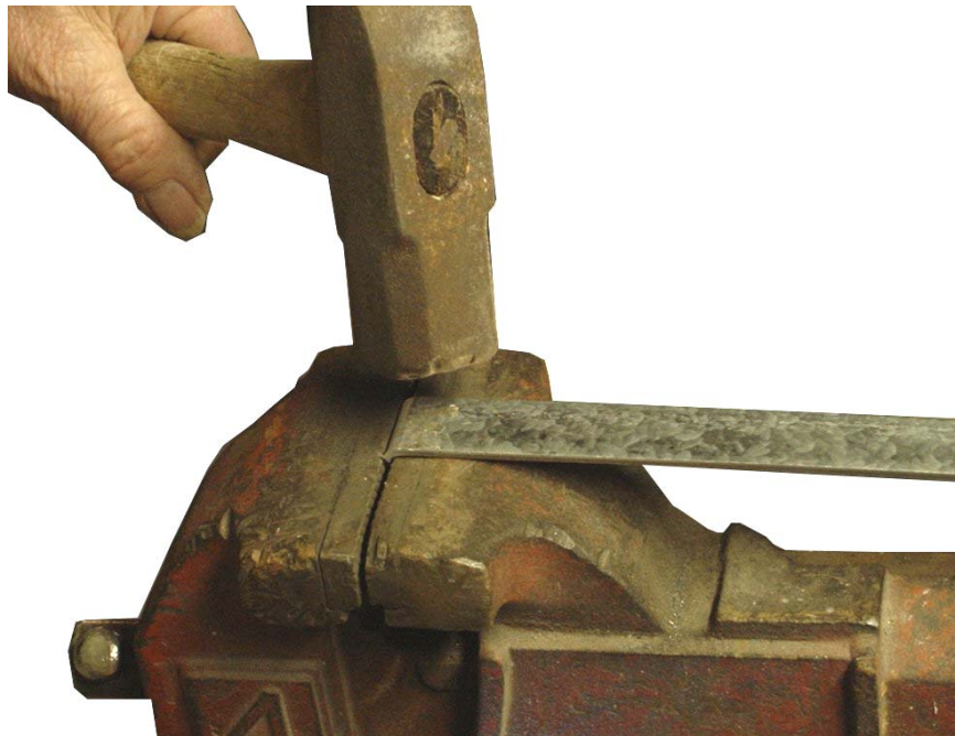
Figure 5 Hammering the bend.
