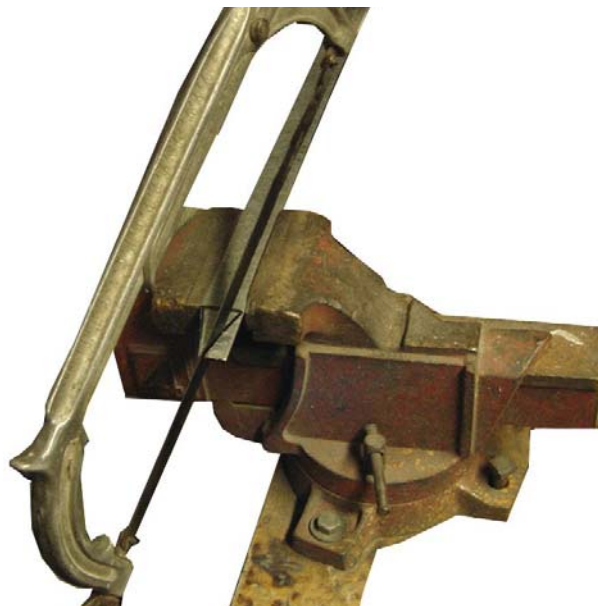
Figure 3 Sawing the iron.
